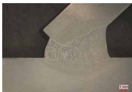
Web plate material thickness 10 mm, included angle 35°
