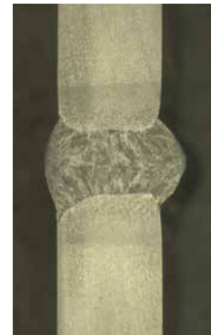
Material thickness 5 mm Air gap 3 mm
