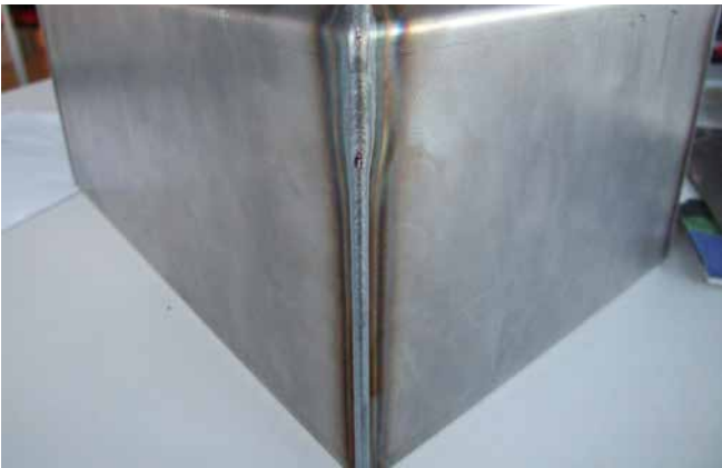
Welding unalloyed sheet metal
