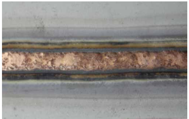
Brazing galvanised sheet metal
