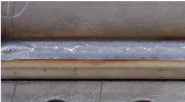
Front view: Lower heat input using forceArc puls ® XQ, less surface oxidation resulting in a better finish
