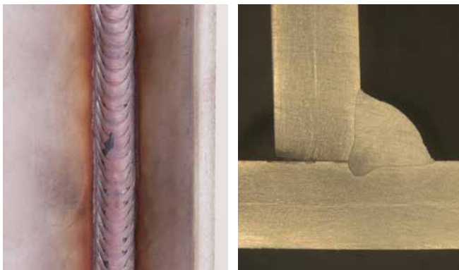
PF Vertical-up weld, straight torch guidance without using the "Christmas tree" technique
