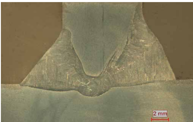
PB Full penetration, welded on both sides
