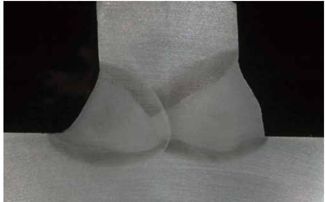
PB Full penetration, welded on both sides
