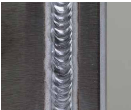
AlMg5, material thickness 4 mm
