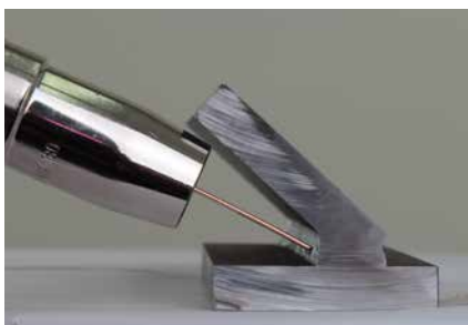
Web plate material thickness 10 mm, included angle 35°
