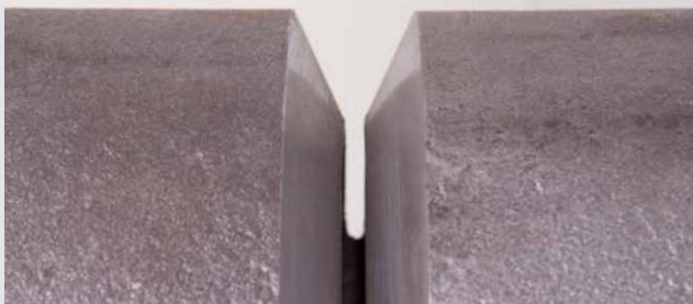
Weld preparation of root welds on pipes, 60° included angle with 3 mm air gap
