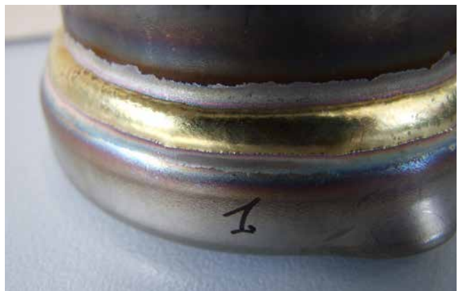
Brazing high-alloy (CrNi) sheet metal
