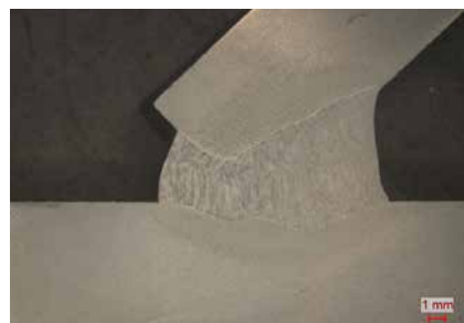
Web plate material thickness 10 mm, included angle 35°
