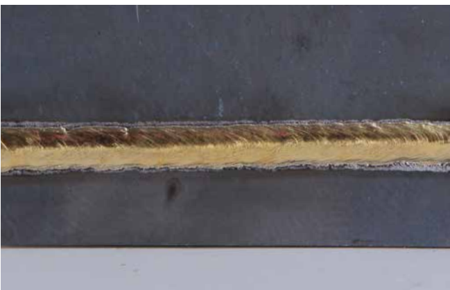
Brazing high tensile sheet metal, e.g. Usibor ®
