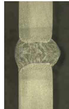
Material thickness 5 mm Air gap 3 mm
