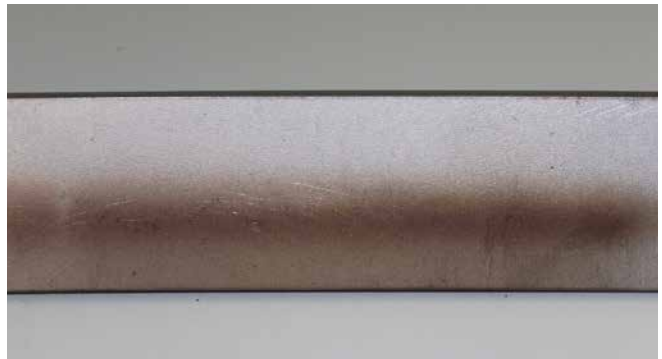
Back view: Low heat input using forceArc puls ® XQ, less surface oxidation
