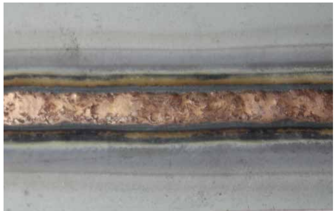
Brazing galvanised sheet metal
