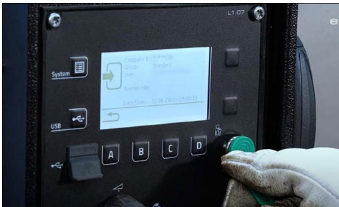
The welder logs on to the welding machine using an RFID key, the Xbutton. Their qualifications are also stored with this key.
