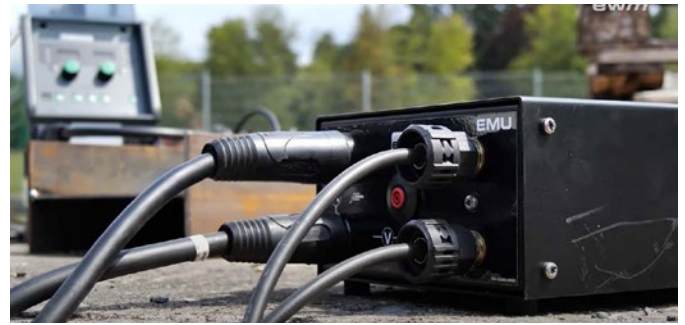
With the Universal logger, welding machines from other manufacturers can also be integrated into ewm Xnet – with the same convenience of simple documentation.
