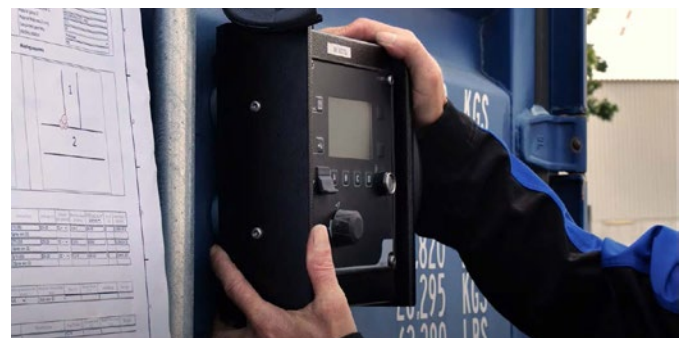
The gateway creates the connection to the ewm Xnet server and establishes the connection to the scanner and the welding machine for data transmission.
