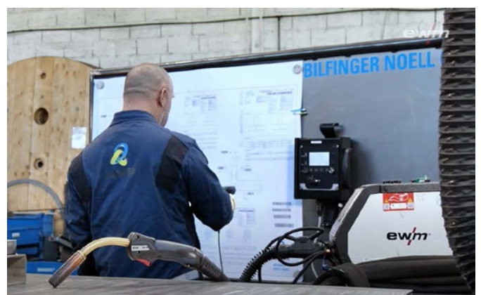
The welder scans the seam to be welded and can then start welding straight away – without any bureaucracy. The parameters are automatically preset on the welding machine.
