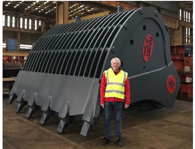
The screening buckets have a volume of 25 m 3 and are used to collect stone and rock from the seafloor while leaving behind any silt.
