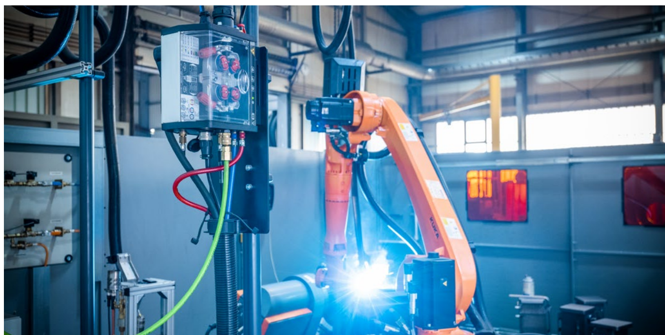
A separate wire feeder ensures reliable transport of the filler material.
