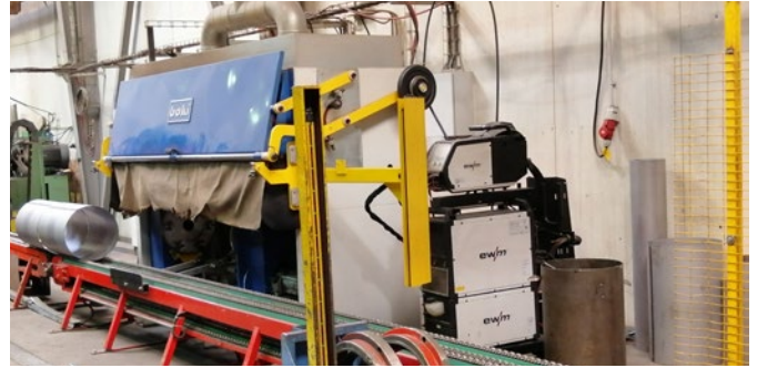
The slip roll machine shapes the pipe, which is then welded directly using the MIG/MAG welding procedure. The wire feeder ensures reliable transport of the welding consumable. The various welding procedures ensure low-spatter seams with a wide range of materials, material thicknesses and diameters.
