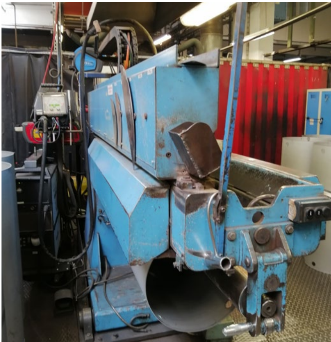
The seam is positioned at the top of the pipe. An axis carries the welding torch directly along the seam from above. The seams are high-quality and low-spatter. The wire feeder ensures reliable transport of the welding consumable.
