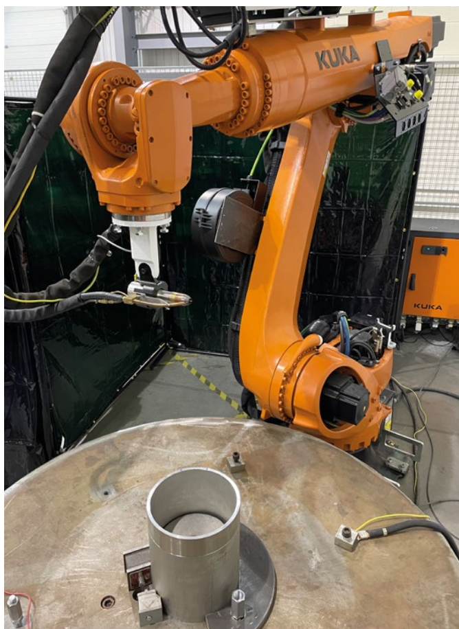
In conjunction with the TANICS™ solution, the welding process forceTig® enables precise, reproducible path guidance of the robot, even with complex seam profiles such as curves.
