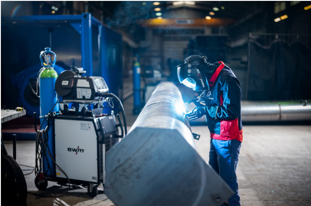
Döpke's wear part assortment also includes suction pipes, which are also welded at the company's halls at the industrial park in Norden, Germany.
