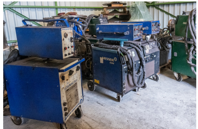
Switching over from step switch controlled Messer-EWM machines to the Titan XQ 350 puls MIG/MAG multi-process welding machine resulted in savings of just under two tonnes of CO 2 per machine, per year.
