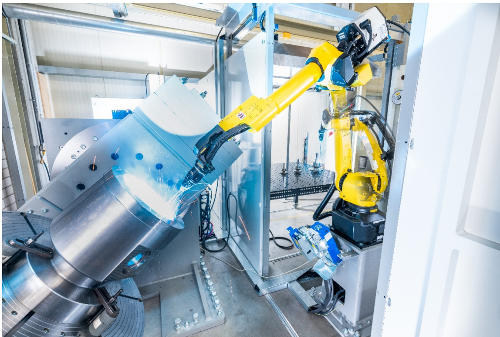
Surfacing of a valve body. The drive 4X wire feeder securely feeds the filler metal on the robot arm.
