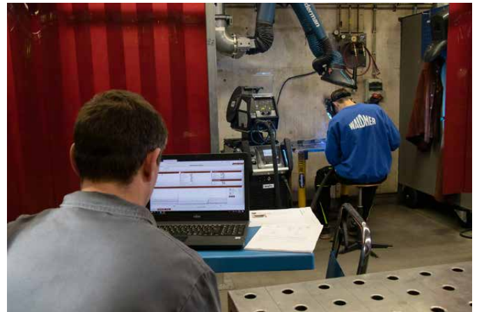
Technology instructor Anton Netzer uses ewm Xnet, the welding quality management system by EWM, for his training. Thanks to welding data collected in real time, he can even see whether the weld seam is ok or not while the students are working.
