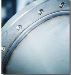
The high-quality seam is applied in a single step and requires absolutely no finishing work
