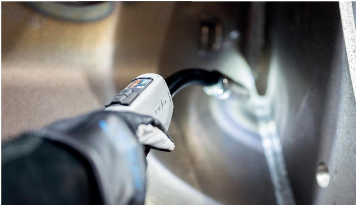
Thanks to the integrated control and graphic display on the RD3X function torch, all the relevant parameters can be set directly on the welding torch. The LED lighting illuminates dark working areas.
