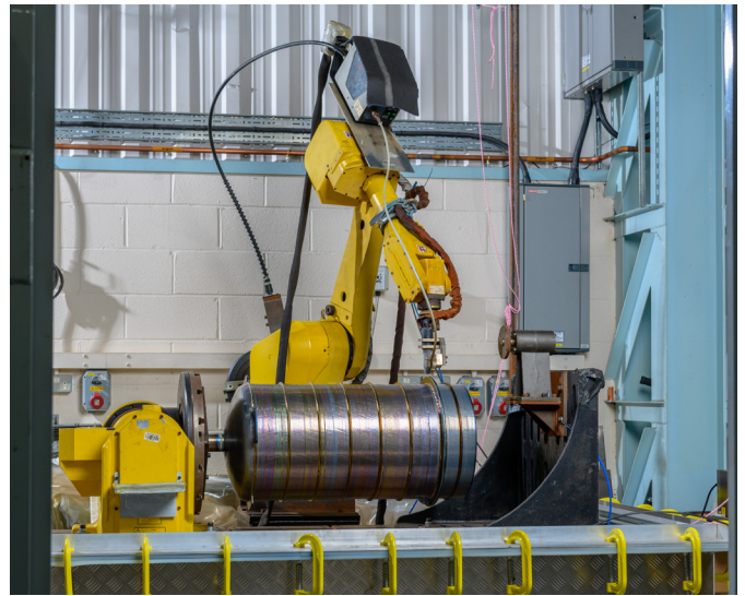
The melted material is applied layer by layer until the component is finished. The entire process is coordinated with robots.
