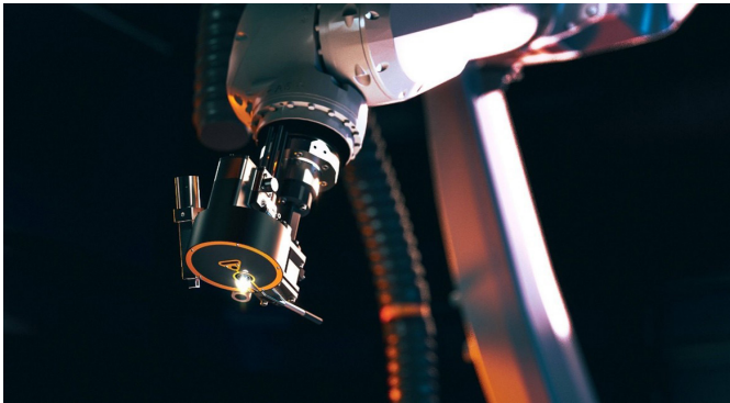
WAAM technology uses the welding arc as an energy source to melt a metal wire.
